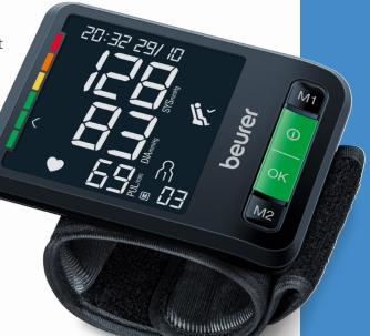
Fully automatic blood pressure and pulse measurement on the wrist With cuff for wrist circumferences from 13,5 - 21,5 cm
