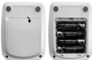
If the battery change icon
