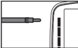
**Important:** This device should only be operated with the original cuff. The cuff included with the device is suitable for an upper arm circumference of 8.7 in - 16.5 in (22 - 42 cm). Replacement cuffs from other models cannot be used with this model. Doing so, will result in inaccurate readings or error messages.
