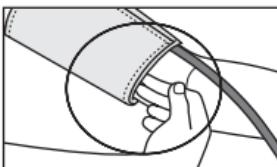
Insert the cuff tubing into the socket for the cuff attachment on the left side of the unit. Make sure it is inserted securely in the main unit and that there are no kinks in the cuff tubing.
