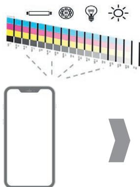
**1.** Camera analyses the colour spectrum of the strips and transforms this into numerical information
